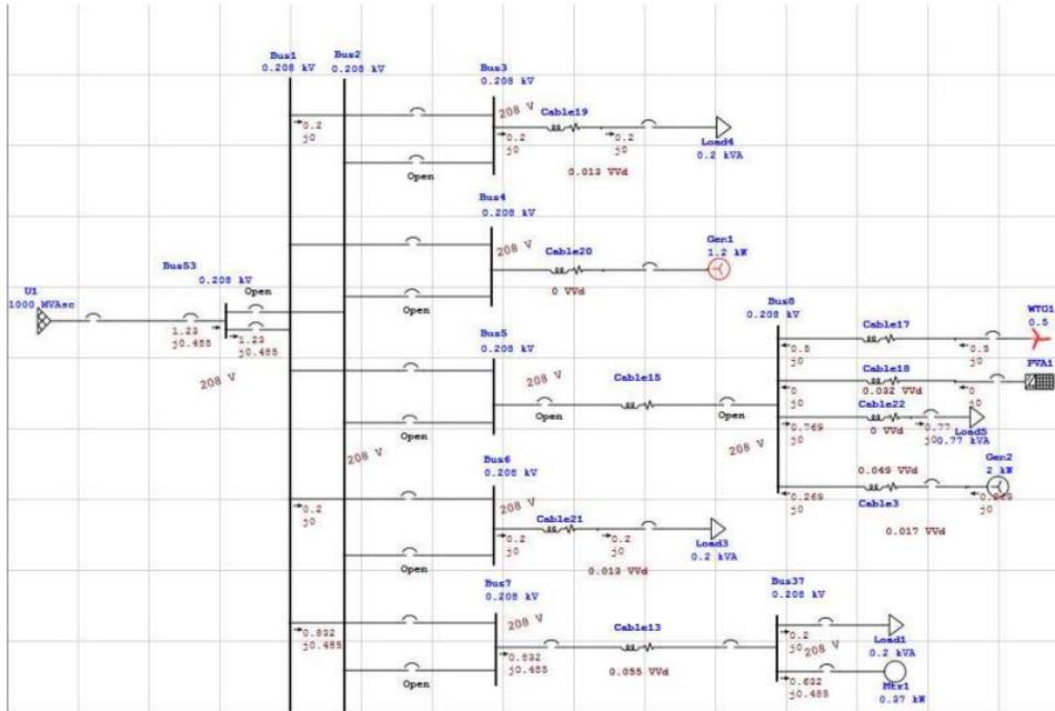
Fig. 1. ETAP® Load Flow study of proposed configuration
